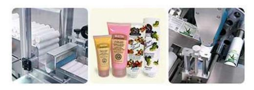
Designed for wrap-around labeling on empty soft tubes. Also applicable for orientation labeling on soft-tubes that have a detectable orientation features. Particularly suitable for the packaging requirements of the cosmetics, personal care and food packaging industries. The fact that the tube body is lack of rigidity and the label is normally very soft and transparent causes new labeling challenges - raised label corners, air bubbles, and tube path blockage ...etc.
