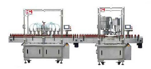
Usage: feeding bottle, linear filling liquid (syrup) in bottle, feeding cap and screw capping.
