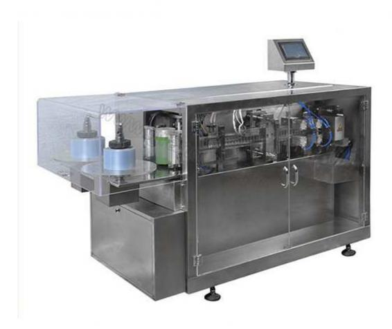
This machine is a kind of compact type liquid filling and sealing machine, it is suitable for small batch filling for different product and widely used for filling oral liquid, perfume, liquid, essential oil, olive oil, health care product etc in pharmaceutical, herbal, pesticide, cosmetic, food and supplement area.
