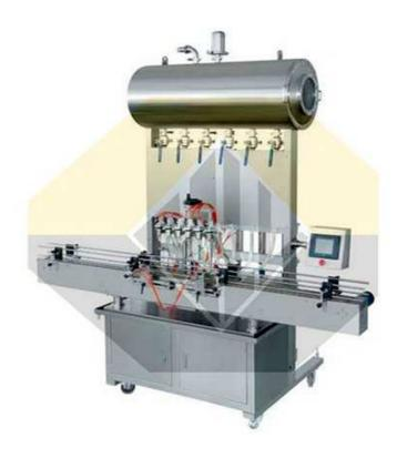
VFJ-6 Automatic 6 Heads (Piston) Jam Filling Machine is widely used for daily chemicals, foodstuffs, pharmaceutics and oil. It can filling various kinds of cream, the filling volumes range is 25-5000ml, the max filling speed can reach 40 bottles/min.
