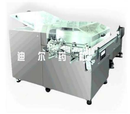
Description: This machine mainly used for plastic bottles automatic collation, orientation and distribution, a variety of plastic bottles filling line of matched products. It can be widely used in pharmaceutical, chemical, food and beverage industry.
