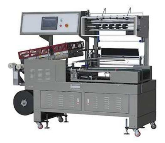
Traditional Middle speed L bar sealer has no reciprocating sealing function, so the sealing line is not strong enough and has the holes or welding seams after shrinking. The new model of TY-703-150-SV is designed to avoid these problems.
