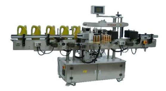
SBM-LM650A is fit for all kinds of bottle. Such as oval shaped, square, flat, and round bottles. It can use both label applicators simultaneously or run individually.
