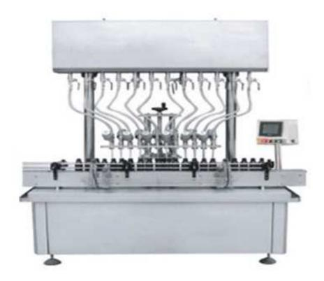
Automatic gravity liquid filling machine adopt logic controller PLC, 6± LCD touch screen system, ordinary pressure flow passage parameters, set the flowing time to control different quantify. It apply to pharmaceutical, foodstuff, pesticide, chemical, etc.
