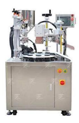
Suitable for plastic tube filling and welding in the field of cosmetic, medicine, commodity, hardware, etc.
