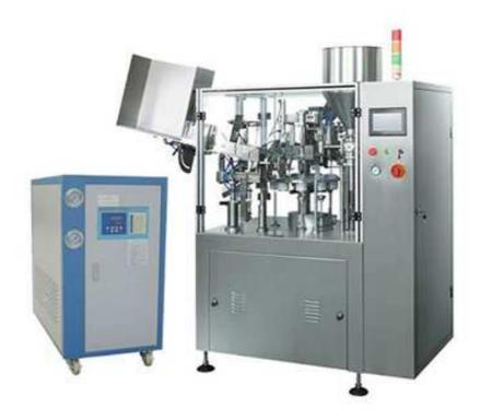
The automatic plastic tube filling and sealing machine is used for filling all kinds of cream products. It's suitable for complex or plastic tubes, sealing and cutting the end of the tube, and printing date on it. Reliable and efficient.
