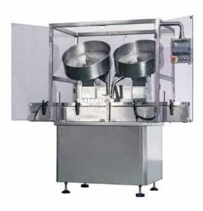
Tablet and capsule counter is designed to adopt unique plate-counting system with a dual-track conveyor on a single frame. The speed up to 60 bpm based on 50 pieces/ bottle. The machine handles a wide variety of tablets, caplets and hard capsules.
