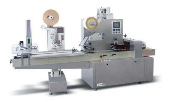
Flow Packing Machine is designed for the second packing of ALU-PVC blister in the pharmaceutical industry, to improve the moisture resistance, and increase the lightproof. This machine adopts PLC to make it programmable. It can equip a coder to print batch number, production date, expiry date and others. This machine can save 20 percent per bag than manual packing machine. With the new ALU-ALU feeder that we designed for all kinds of tablets, our machine can be a truly automatic packing machine.
