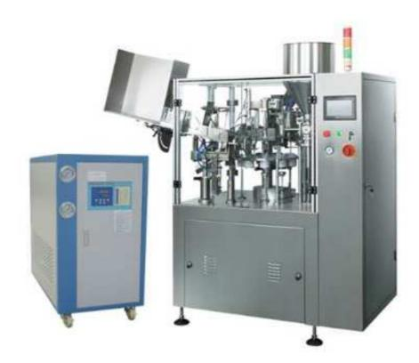
The automatic plastic tube filling and sealing machine is used for filling all kinds of fluid material into complex or plastic tubes, sealing and cutting the end of the tubes, and printing date or series numbers on the end. Automatic Plastic tube filling and sealing machine is widely applied to daily chemical, pharmaceutics, food, chemistry industry, etc
