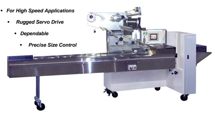
Designed for high speed, multi-shift operations, the Model 3500 horizontal wrapper is the ideal choice where performance and reliability are required. Constructed with a heavy duty modular frame, this machine is equally at home as a basic wrapper or as a high speed wrapper with fully automatic product feeders operating at very high speeds. The wrapper accommodates a wide range of heat sealable wrapping materials, from standard single layer films to multiple layer laminations.
