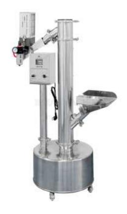
LSV-C100 Capsule Polisher has achieved double functions of capsule polishing and elevating. Inlet of the machine can be connected with any model of capsule filling machine, and outlet with capsule sorter and metal detector, so that to realize the production line of capsule polishing, elevating, sorting and detecting.
