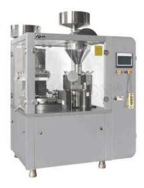
NJP-3000D automatic capsule filler processes the products for optimal productivity up to 3000 capsules per minutes, featuring low-maintenance operation, minimal downtime, and overall dependable production.
