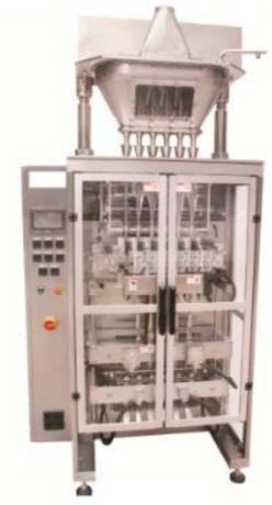
Stick pack machines are a specific type of vertical form fill seal machines which allow for the quick and efficient filling of stick pouches, which are ideally suited for coffee, drink mixes, and various liquids and gels. Additional specifications on sachet machines and vertical form fill seal machines in general are provided separately.
