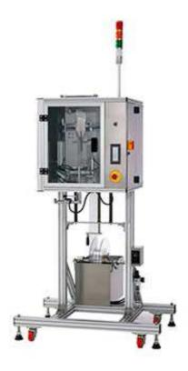
Tamper Evident Band Applicator, CH-100 is designed with SUS frame to match production requirement of Foods & Pharmaceutical industries. Modularized machine body & assemblies for quick adjustment & parts change. Cutting Unit is designed with quick change feature to save changing time of cutting blade. Also, machine could be installed remote control feature to monitor production.
