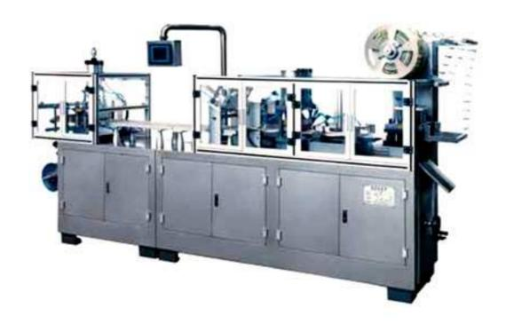
This blister packing machine which is suitable for "PVC/PET blister + Card" packaging for such as battery, glue, lipstick, pen, injection, toy gun, buring torch, toy car, scissor, alarm, toothbrush, coat & hat hooks, chopsticks, cleaning balls, bottle openers and so on.
