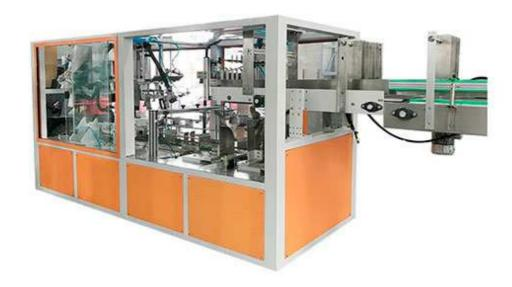
The machine adopt to servo location, PLC controlling, auto operation, main drive adopt to import motor drive, multi degree rotation via chain, chain wheel speed regulator ect. It auto degree is high, reliable controlling, easy to adjust, intelligentize manipulation ect advantage, can widely used for beverage, beer, chemistry, food, medicine ect industry, can do all kind of tin and bottle second time package, can match with auto filling production line.
