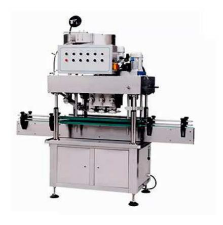
This machine is suitable for various bottles shapes. When it needs to replace bottle or cap, you only adjust the position of the parts, no need to replace any accessories, and it will not be screwing caps if it is without bottles during the capping process. The cover lid assortment, the screwing cap and the clipping bottle speed can be respectively frequency-adjusted and adjusted to meet the screw caps of various specifications within the specified range.
