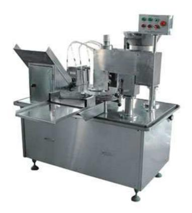
As the main device of the oral liquid production line, this oral liquid filling and sealing machine is specially designed for filling, capping, and sealing 5-30ml vertical bottles with easy open lids or aluminum-plastic lids.
