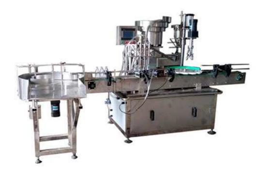
Adopts the positive displacement ceramic pump or stainless-steel pump for filling, with high precision and wide range of dosage.
