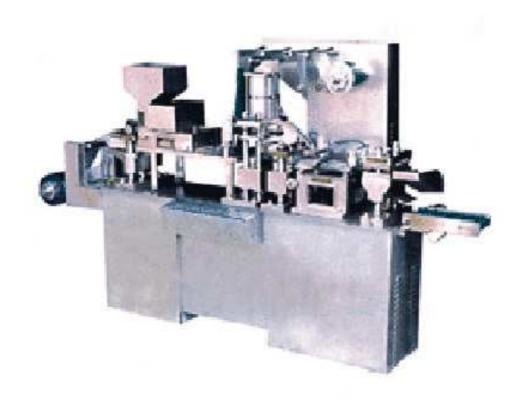
DPP Series Plate Type Blister Packing Machine incorporates the functions such as heating by contacting with the flat plate, cap shaping on the flat plate under positive air pressure, sealing by means of the flat and heated plate, batch number embossing and cutting by punching. It features solid and caps in beautiful appearance as well as convenient in operation and maintenance.
