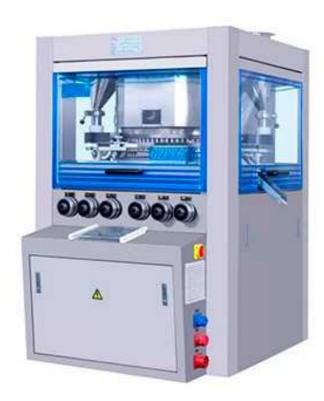
This machine is one kind of double side rotary tablet press machine, which can press granular materials into round shape tablet, irregular tablet or double-side engraved tablet.
