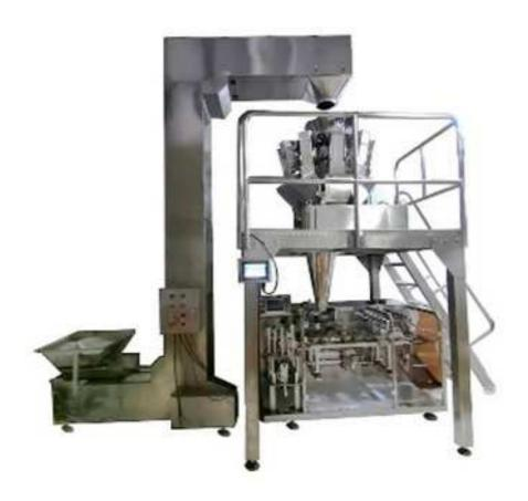
The premade bag automatic packaging machine replaces manual packaging, and realizes packaging automation for large enterprises and small and medium-sized enterprises. The operator only needs to put the finished bags one by one, and put hundreds of bags in the bag removal department of the equipment at a time. The mechanical claw of the equipment will automatically take the bag, print the date, open the bag, give a signal to the measuring device, and blank, seal, and output.
