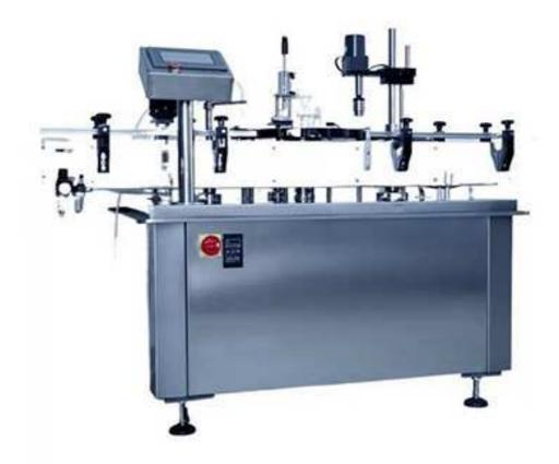
This machine is the main machine of filling and capping in liquid production line, mainly used for filling, capping and capping of glass bottles or plastic bottles.
