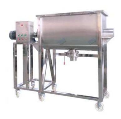
Dry food mixer is a new design and upgraded equipment in food dry powder processing and production, which can help uniform mixing all kinds of dry food powder with good properties of liquidity, such as flour powder, milk powder, coffee powder, etc.
