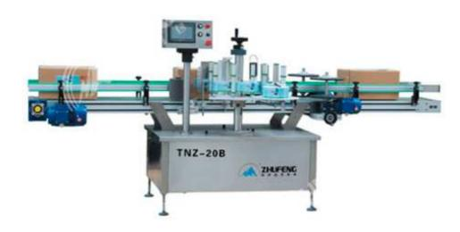
This machine is mainly used for the finished carton side or flat adhesive paste, the whole machine adopts 304 Stainless Steel and aluminum alloy materials, PLC program control, photoelectric detection, sending label & labeling. The label is smooth and accurate, simple operation and maintenance, can be used with filling production line.
