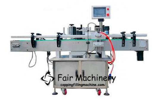
For the pharmaceutical, food, cosmetic and other industries round bottle labeling, can be affixed to the week and semicircular labeling labeling. Optional automatic turntable Unscrambler can be directly connected to the front end production line, automatic feeding bottle into the labeling machine, increasing efficiency. Optional configurations ribbon coding labeling machines, online print production date and batch number, reduce bottle packaging processes, and improve production efficiency.
