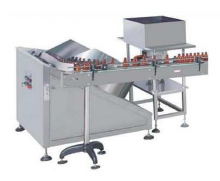
This machine is suitable to round bottle, flat bottle, automatic feed bottles to sorting plate by elevator hopper, then bottle will be unscrambled upright onto the conveyor. It greatly reduced the labor intensity.
