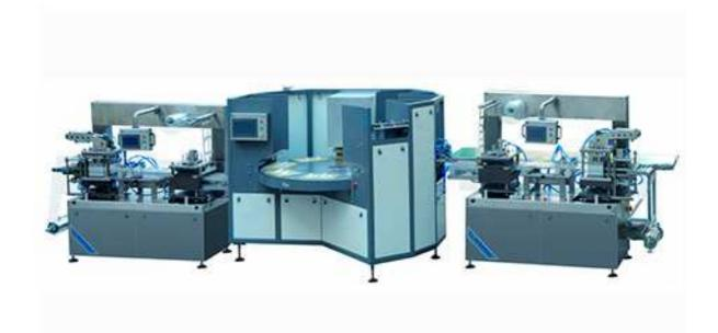
The Automatic Impulse Blister Sealing Packing Machine is used for double blisters packaging, blister to card packaging, card to card packaging. Because the product is so visible, the packaging is so popular with manufactures and consumers.
