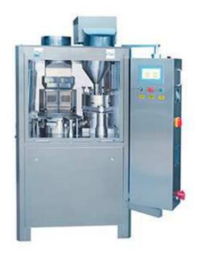
This machine is designed to meet the needs of mass production on the basis of NJP-1200 automatic capsule filling machine. Its function has reached the domestic advanced level, and it is currently the most ideal equipment for the production of capsule drugs in the pharmaceutical industry.
