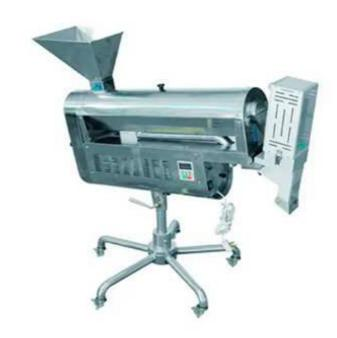
This machine is a newly designed Capsule Polisher to polish capsules and tablets, it is a must for any company producing hard gelatin capsules.
