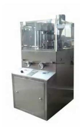
The tablet press, Mini in size and Single Rotary is an ideal choice for R&D work as well as small scale productions. It is also used to avoid wastage when high value ingredients are used for tablet formulations, also known as lab tablet press. The mini tablet press is designed with GMP considerations. It is sturdy, fitted with single sided turret of special grade Iron Casting.
