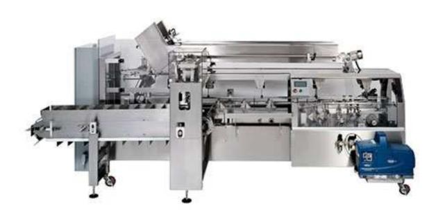
The HC-3200 is a high-quality, automatic cartoner that erects, closes, glues cartons and inserts the product into the cartons. The automatic loading of the product is accomplished with the addition of a servo-controlled, cam-driven product inserter to a cartoner built on the basic foundation of the HC-120 semi-automatic cartoner. The cartoner is constructed of stainless steel and anodized aluminium.
