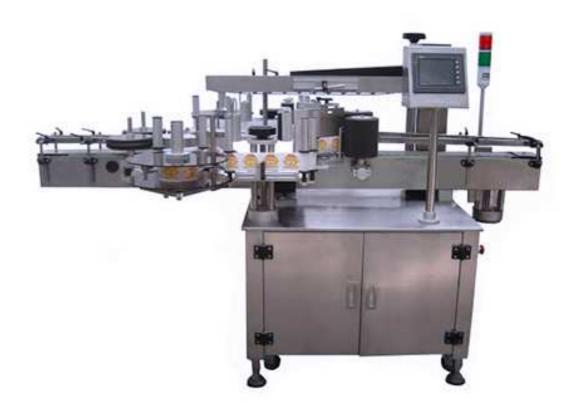
This machine is applied to label the self-adhesive label on various cylindrical bottles, flat bottles, Square bottles. Suitable for double side and single side labeling.
