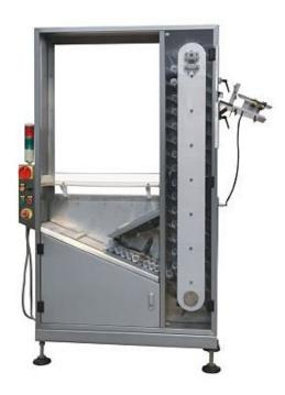
ZH-200 automatic tube feeding machine is generally used with tube filling and sealing machine to achieve sound performance. It is manufactured with advanced European technology and has been acknowledged by CE and SGS. The feeding capacity of such tuloader is 30 to 200 tubes in one minute. It can support 650 to 1000 tubes. The suitable tube length varies from 13.5 mm to 60 mm and diameter is from 60 to 1000.
