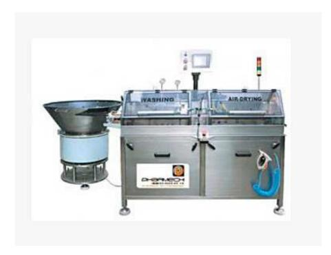
We are offering Rubber Stopper Washing Machine. This microprocessor controlled Washing Machine is used for washing Stopper gently with the help of air fluidization without generation of particles.
