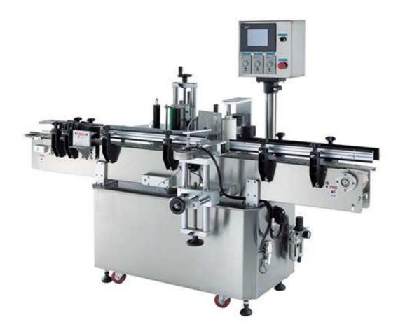
The machine is designed for partial/fully wrap-around labeling on round containers. Available for positioning labeling for round bottles with a handle. Available to apply one or two labels at a time on the bottle.
