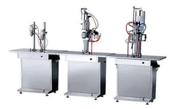
JF-QGB semi-automatic aerosol filling line, composed of semi-automatic double-headed filling machine, semi-automatic sealing machine, semi-automatic inflator (propellant filling machine (including booster pump)) three parts. The user can assemble the production line according to the process of aerosol product.
