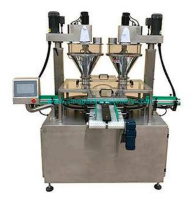
This series could do work of measuring, can holding, and filling, etc, it can constitute the whole set can filling work line with other related machines, and suitable for filling kohl, glitter powder, pepper, cayenne pepper, milk powder, rice flour, albumen powder, soy milk powder, coffee powder, medicine powder ,additive, essence and spice, etc.
