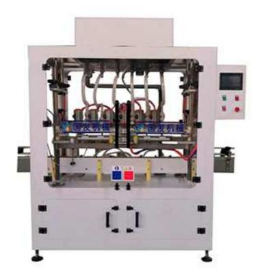
GFZLQ automatic antiseptic gravity filling machine can be used for filling various acidic or alkaline liquids such as toilet cleaner, kitchen oil remover, laundry detergent, hand sanitizer, etc.
