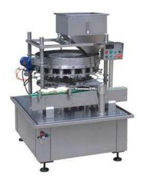
This is the latest granules/beans/grains filling machine which designed and produced on the basis of similar machines at home and aboard. It is high capacity (18/36 filling heads for option), running steady, no-can-no-granules, and it will stop if the machine goes backward when empty cans enter into it, alarms while malfunction happens.
