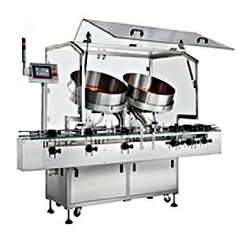
Being widely used for the filling and packaging of the tablets, pills, granules, hard capsules, soft capsules and irregular slices in the pharmaceutical, food and chemical industries, the automatic double-head tablet counting machine can carry out the operations of rearranging and feeding bottles, correct counting tablets by two heads and filling various granules with different shapes into bottles.
