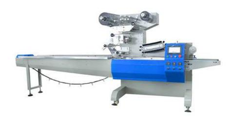
High Speed hffs flow pack pillow packing machine is suitable for packing regular products that need high speed and high efficiency. Such as small candy, chocolate bar, single biscuit / cookies, soap bar, etc.
