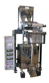
The MK-215 is a fully pneumatic vertical form fill and seal packaging machine designed to package various snack products. This Vertical (VFFS) form fill seal packaging machine uses linear weigh filler system to produce center sealed, 3 side sealed and 4 side sealed pouches / bags.
