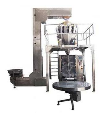
This box-type bag packaging machine is a latest type developed by our company; four corners are added on the packaging bag based on vertical bag, making the packaging bag have a stronger spatial vision, nicer appearance and more attraction.
