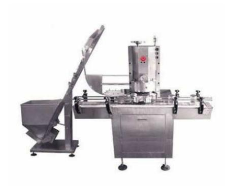
This machine adopts the high efficiency sealed vacuum chamber structure; Vacuum degree can be set as required. Can feeder the bottle automatic, make vacuum automatic, automatic capping, automatic bottle out. This machine applies for condiment, honey, oil, wine industries of the shaped glass screwing bottle automatic pumping sealing.
