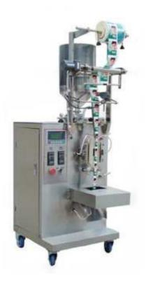
This stick machine can automatic measuring, making bag, filling, sealing, cutting off, batching number and output counting, suitable for viscous material such as honey, chocolate paste, etc.
